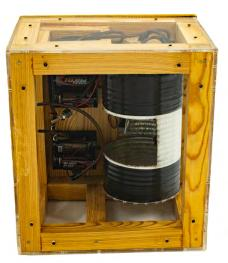
a 7.5 inch by 4-inch diameter metal can, four "C" cell batteries, a barometric pressure switch, and a "loop" switch. The bomb failed to detonate because it contained barium nitrate, a powder often used to create green smoke in fireworks, not explosive powder. The device burned in the cargo compartment causing the aircraft to make an emergency landing at Dulles International Airport outside Washington, D.C. due to dense, green, smoke.
